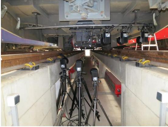
*Fig. 9: Stationary and moving system of cameras*
