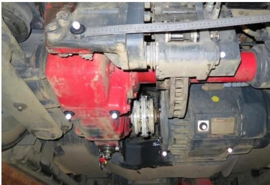
*Fig. 7: Markers of the system Qualisys placed the gearbox and the asynchronous motor*
