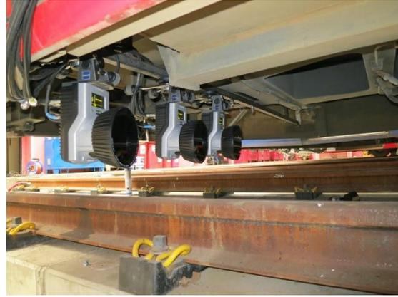
*Fig. 10: Moving system of cameras mounted to the holder*
