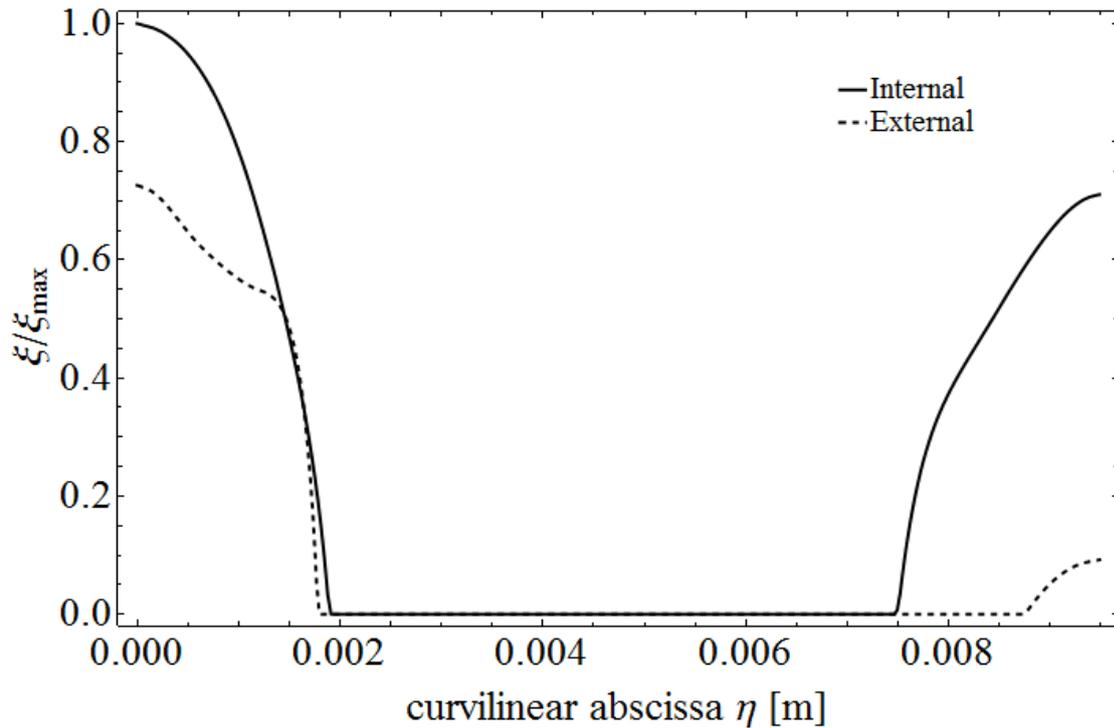
Fig. 4. Distribution of martensitic phase along the curvilinear abscissa  $\eta$  (external and internal side, see Fig.3.)
